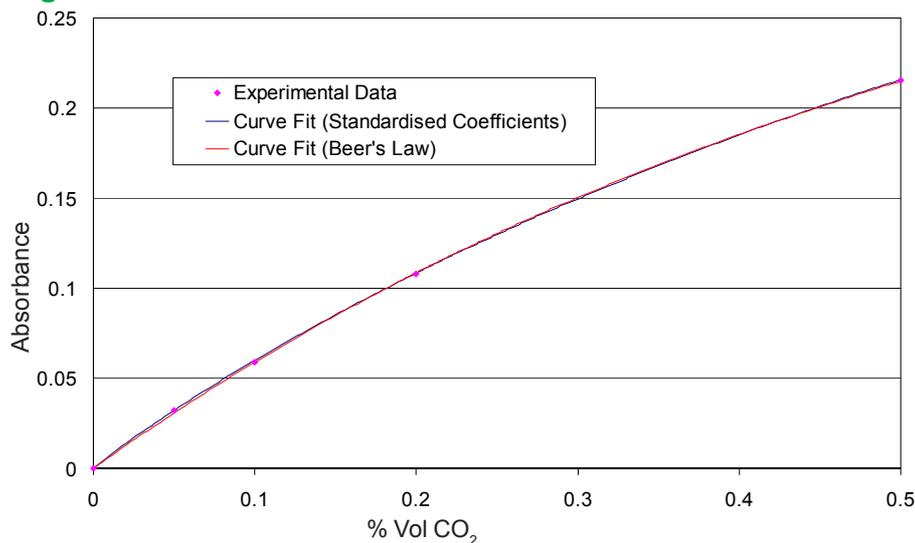
Typical response from 0 to 5000ppm CO<sub>2</sub>.
