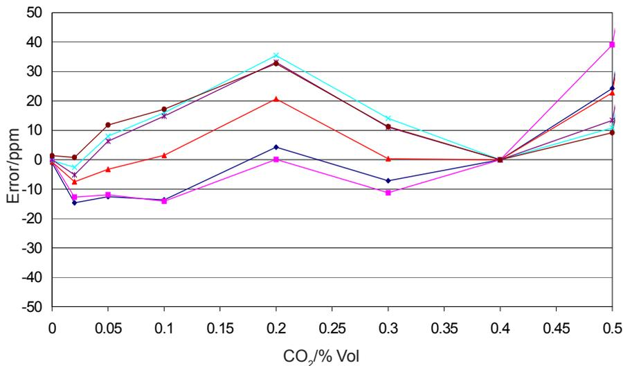
Custom linearisation is not necessary with the IRC-A1. Using universal linearisation constants, repeatability between cells is very good, allowing easy implementation.
