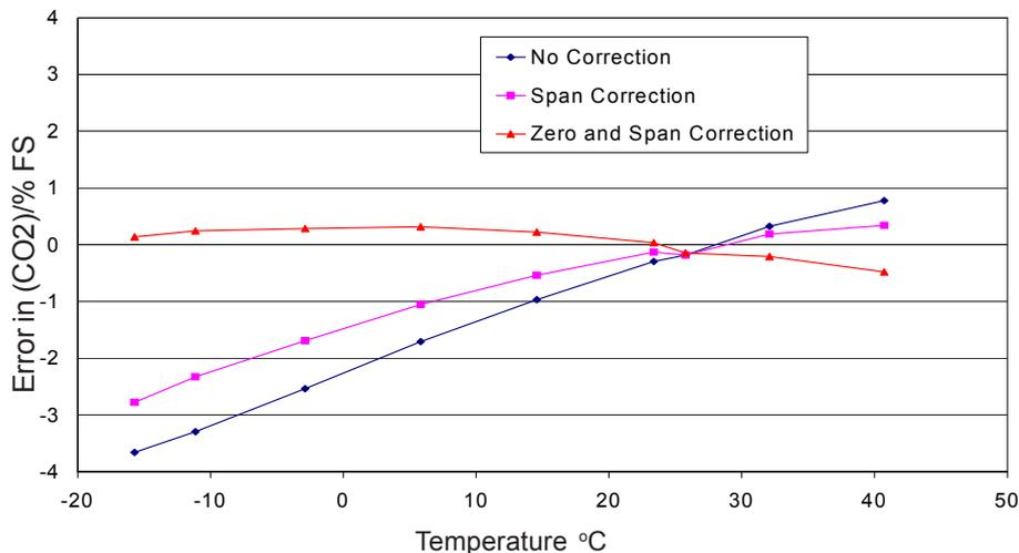
Temperature compensation corrects for temperature error in the detector.
