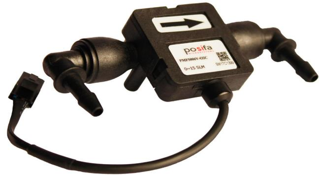
PMF5006 features Posifa's third-generation thermal flow die, benefiting from the latest innovations in microfabrication. The sensor die uses a pair of thermopiles to detect changes in temperature gradient caused by mass flow, delivering excellent signal-to-noise, and repeatability. The "solid state" thermal isolation structure on the sensor die eliminates the need for surface cavity or fragile membrane used in competing technologies, making the sensor resistant to clogging and pressure shock.
